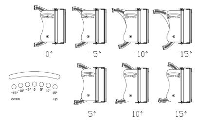
**5c) SECURE THE ANGLE SETTING** -- Once the angle has been chosen, tighten both bolts with hardware provided.
