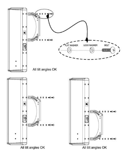
**3b) CBT 100LA-1** -- Mount the **SPEAKER BRACKET** to the speaker with the provided M6-15L hardware. For the CBT 100LA-1 there are seven (7) possible mounting position. Choose the one that best suits the application. Be sure the hook feature of the **SPEAKER BRACKET** is downward.
