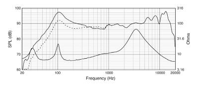
On-axis in half-space (2pi, solid line) and full-space (4pi, dotted line) at thru (8 $\Omega$ ) setting; input impedance (lower solid line)
